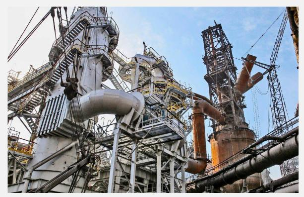
Over 950 tons of steel structures, equipment, pipeline of gas purifiers and deduster were fabricated and installed, including steel structures of deduster, scrubber, water separator, large diameter pipelines, supporting structures, platforms and stair shafts.
