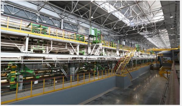
Full scope of construction and assembly works was performed for continuous pickling unit No.4 (NTA-4), along with hydrochloric regeneration unit, reverse osmosis system and butt-welding machine installation.
